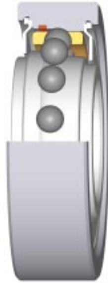
Dry Pump Bearing with Grease Reservoir
