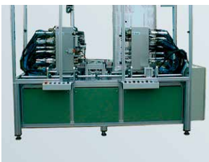
23 placing heads to assemble a computer chassis
