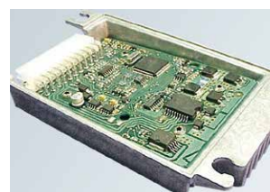
Automotive die-cast chassis with PCB
