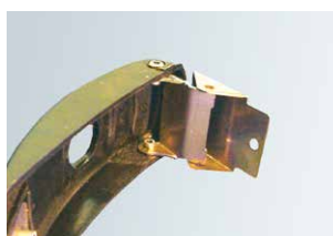
Composite material latch for wheel cover
