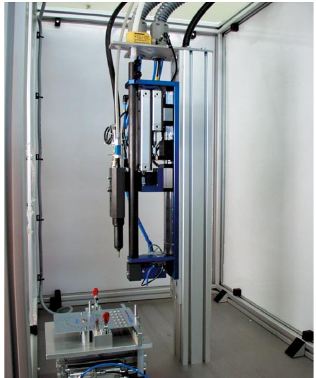
Autoload MK4 for automatic loading of Speed Fastening® handtools
