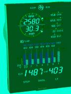
Now you can be sure that you are within the **horsepower limits** of your engine. At the present time HorsePower is only available on single engine 4 and 6 cylinder instruments.
